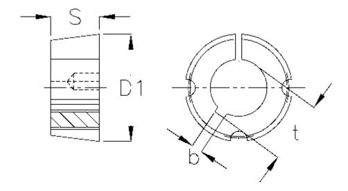
b = 6 Bore = 22 Bush type = 2517 D1 = 85,5 S = 44,5 Screw size =  $1/2 \times 1$ " t = 24.8 Transmission moment = 1310
